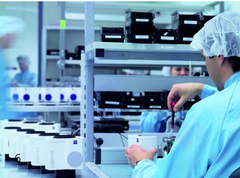
1. Before the assembly begins each lens is exactly calibrated against a "0-lens type". This lens value is digitally saved in a data pool – the basis on which computer-calculated combinations are established. By doing this, an optimally coordinated lens family is developed for every individual microscope
